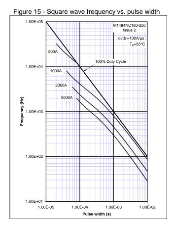
Figure 16 - Square wave frequency vs. pulse width
