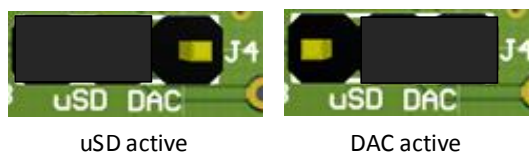
Figure 7: DAC/μSD J4 jumper.
