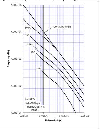
Figure 15 - Square wave frequency ratings
