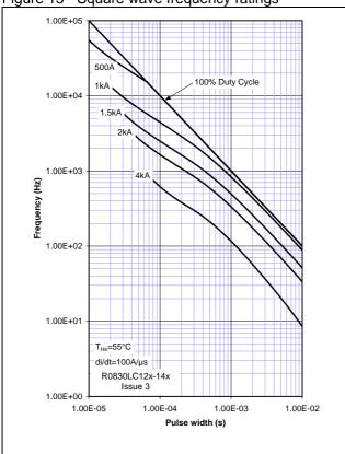
Figure 14 - Square wave frequency ratings
