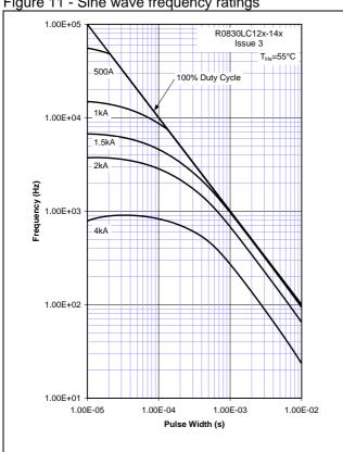
Figure 12 - Sine wave frequency ratings
