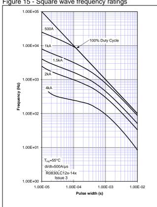
Figure 16 - Square wave frequency ratings
