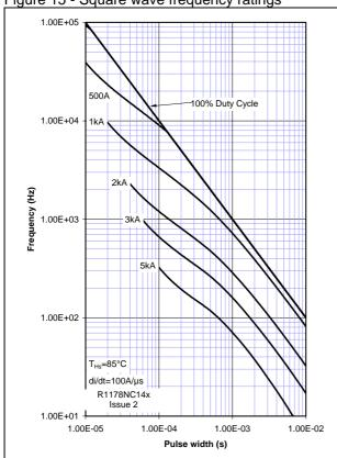
Figure 16 - Square wave frequency ratings
