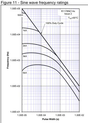
Figure 12 - Sine wave frequency ratings
