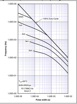
Figure 15 - Square wave frequency ratings
