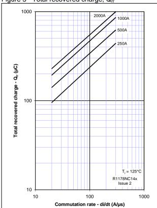
Figure 6 - Recovered charge, Q<sub>ra</sub> (50% chord)
