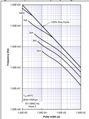
Figure 14 - Square wave frequency ratings
