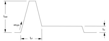
The magnitude of  $I_{GM}$  should be between five and ten times  $I_{GT}$ , which is shown on page 2. Its duration  $(t_{p1})$  should be 20µs or sufficient to allow the anode current to reach ten times  $I_L$ , whichever is greater. Otherwise, an increase in pulse current could be needed to supply the necessary charge to trigger. The 'back-porch' current  $I_G$  should remain flowing for the same duration as the anode current and have a magnitude in the order of 1.5 times  $I_{GT}$ .
