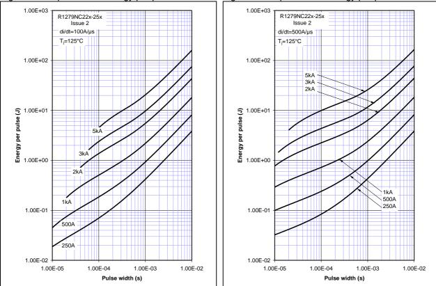
Figure 17 - Square wave energy per pulse
