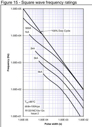
Figure 16 - Square wave frequency ratings
