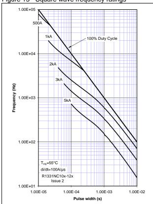
Figure 14 - Square wave frequency ratings
