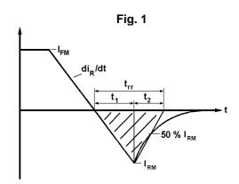
(ii)  $Q_{\text{rr}}$  is based on a  $150\mu s$  integration time i.e.
